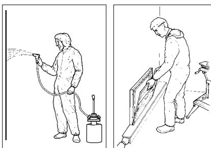
Paint or cover the damaged area, see a8 and a16
