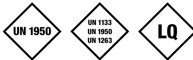
**Figure 1** Examples of limited quantity marks
