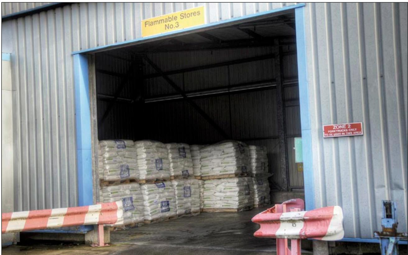
**Figure 31** Segregated and banded chemical storage area
